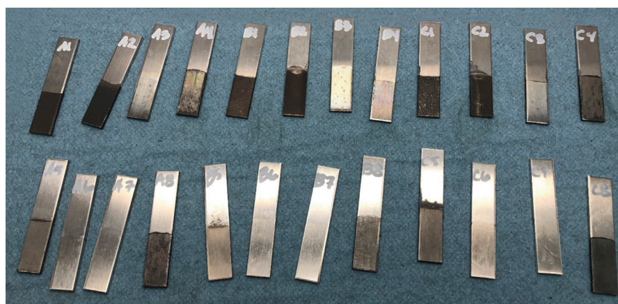
Figure 2. Staining/corrosion/pitting is observed from aluminum coupons soaked in metalworking fluid diluted to between 3% and 5% in 20 dh (approximately 350 ppm) hard water at 50 C for 18 hours. (Figure courtesy of Clariant.)
